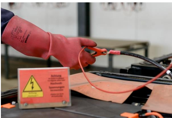
Photo 3: Large batteries such as electric vehicle battery have to be discharged. Photograph rights: REDUX/Schimanke.
